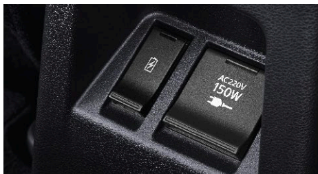
AC POWER OUTLET 220V/150W 1
